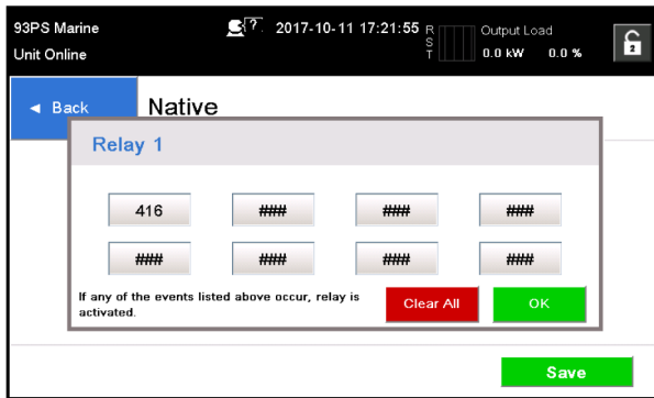
Figure 29. Entering the codes of the functions that will trigger the relay
