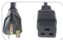
010-9337: 6-20P to C19 250V, 20A straight blade 8-foot, 12 AWG/3-wire
